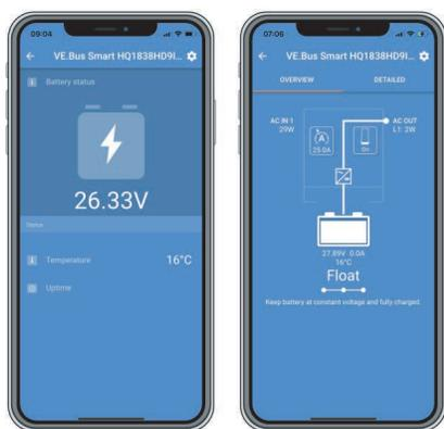
VictronConnect screens without and with inverter/charger connected.
