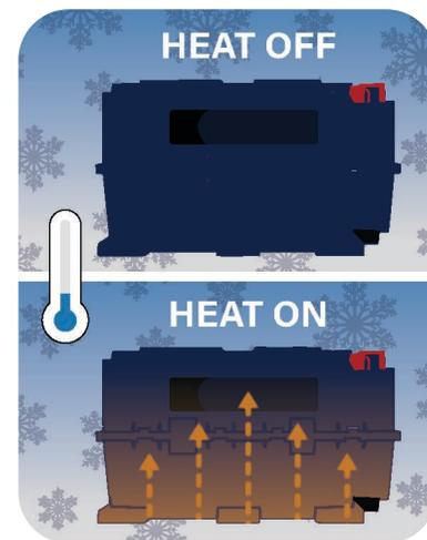
The heaters draw 1.8 amps (per battery) of power and typically run on a 30% duty cycle. This means at 0°F, the heaters will be on 30% of the time, and off 70% of the time. That means if it is cold, we can expect 0.6 Ah of energy (per battery) to be used to keep the batteries at proper charging temperatures.
