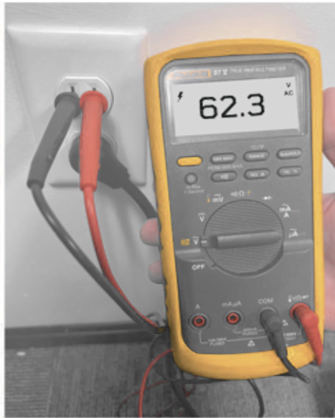
Figure A - Low Voltage
