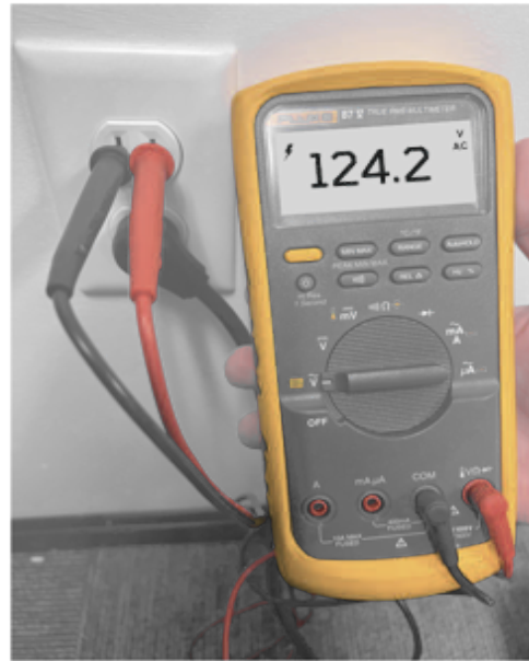
Figure B - Correct Voltage
