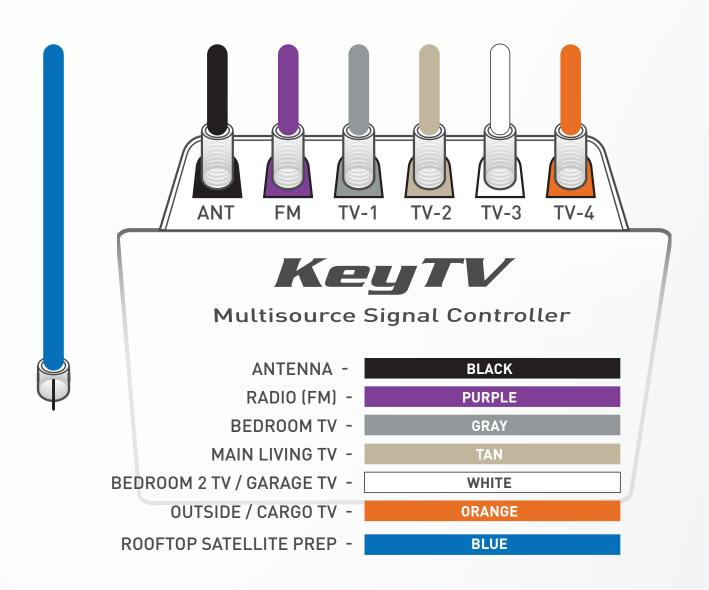
Applications with 5 TV locations require the replacement of the factory installed splitter located between TV 4 & TV 5 with an approved satellite providers splitter.
